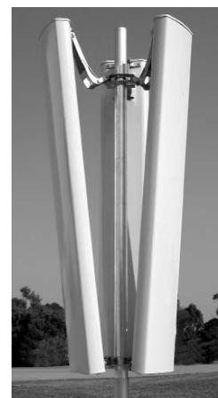
Dualband Antenna at 5deg tilt using APM70-3C plus optional APM40-E1 and APM40-E2 mounting kits
