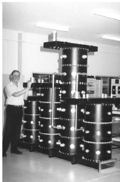
Waveguide Directional Combiner for Ch 28 29, 31 and 35 featuring 3-pole, 4-pole and 6-pole modules
