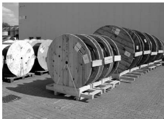
Drums packed on pallets with reduced protection
