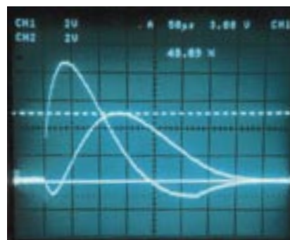
CENTER Here the center conductor's peak is only 48.89% of the total. Note that the area under both waveforms is nearly equal. Each has 50% of the total surge energy.
