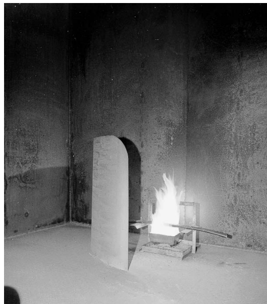
Test IEC 61 034, low smoke.
