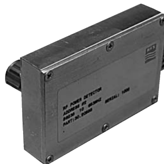
Wideband RF detector module.
